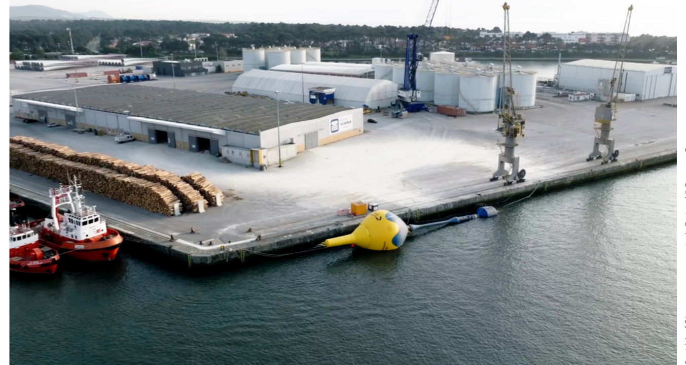
Sea trials of C4 wave energy converter in Portugal © CorPower Ocean
