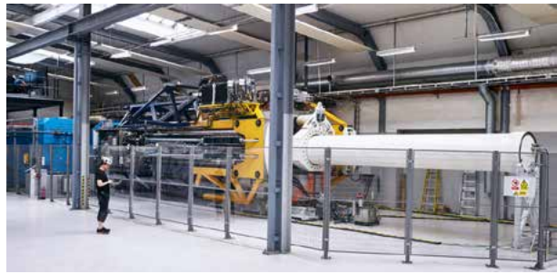
Corpower C4 PTO in dry-test rig in Stockholm. © Corpower
