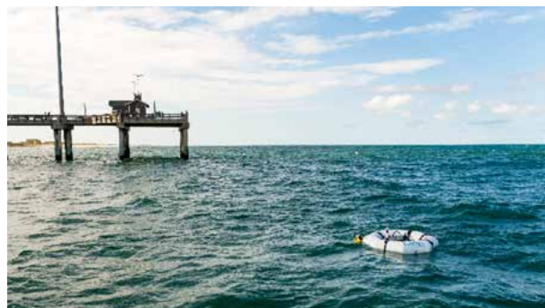
NREL's HERO WEC device is taken out for an ocean deployment in August 2022 off the coast of Nags Head, North Carolina, with the help of the Coastal Studies Institute. © Coastal Studies Institute
