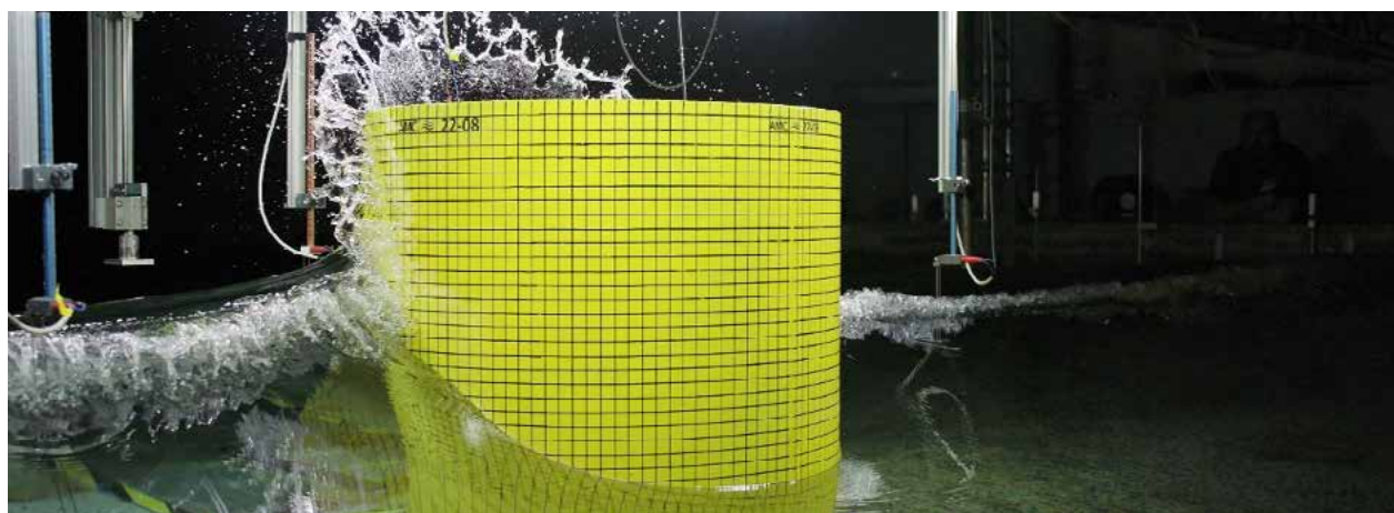
Focused wave slamming on a fixed offshore wind turbine model in the AMC wave basin
