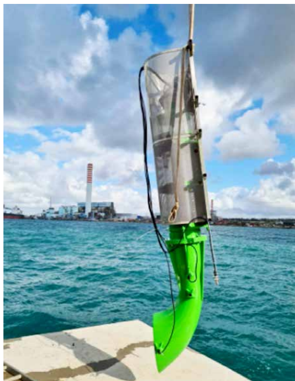
The WAVESAX 1:5 scale prototype and installation in the port of Civitavecchia
