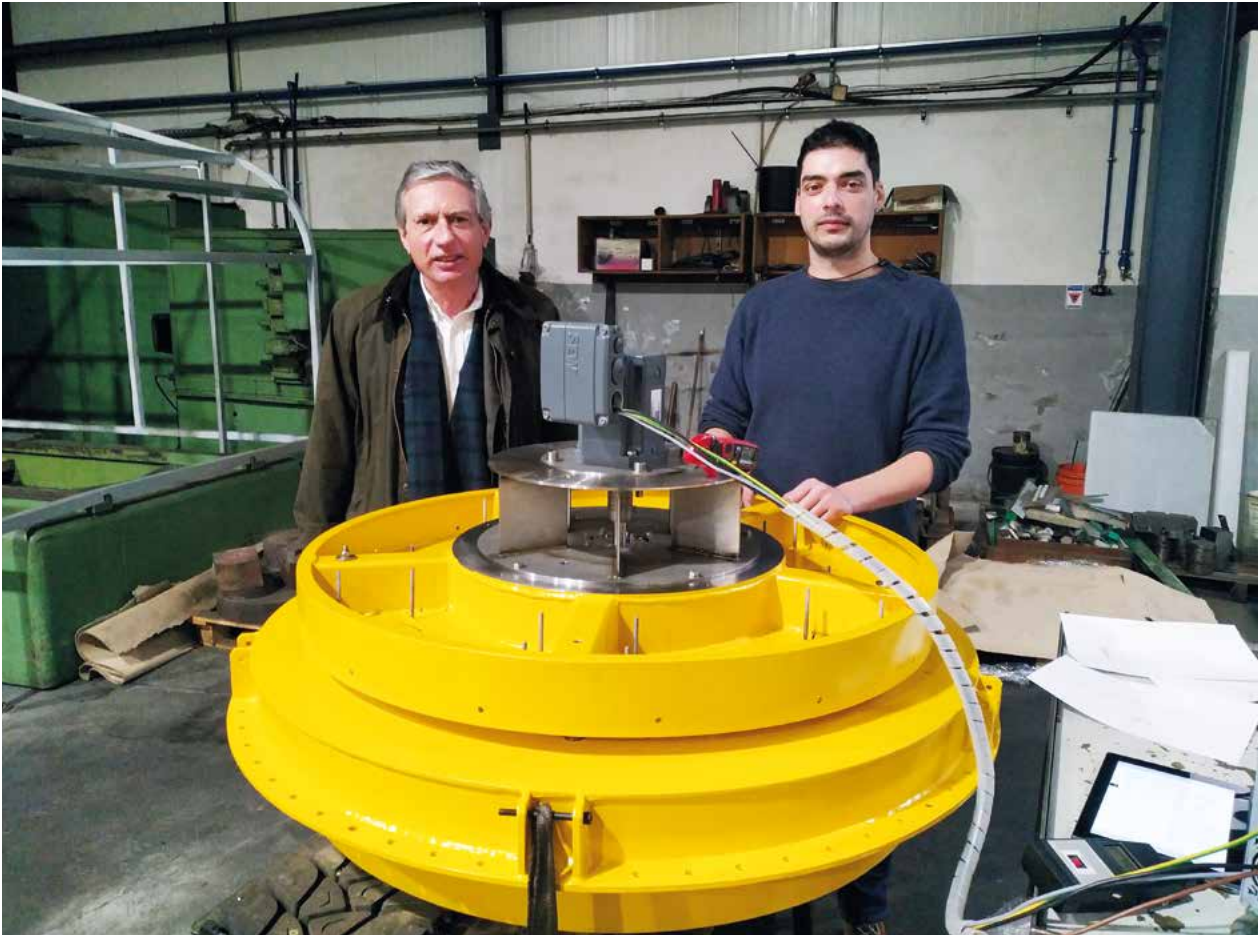
2.2 kW PTO system for off-grid OWC wave energy converter at IST
