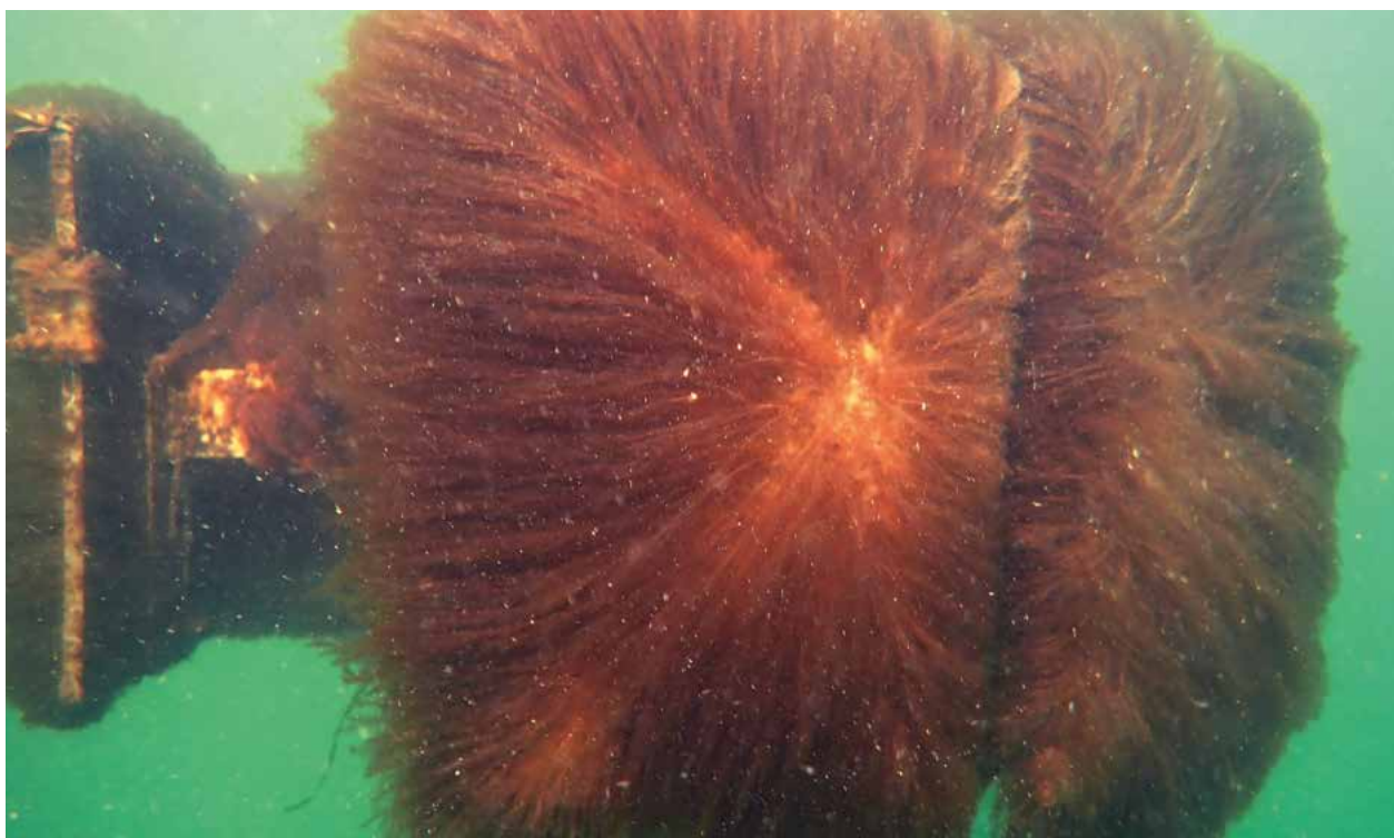
Biofouling plates for growth rate assessment during the Element project in ria d'Etal. © France Energies Marines
