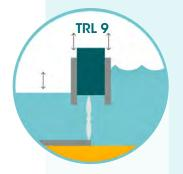
Barrage Water that entered an enclosed tidal basin with high tide is released in low tide and generates electricity by passing through turbines.
