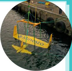
Minesto kites look like little submarine planes, a resemblance that comes from the company's origin as a spin-off of an aircraft manufacturer. Due to their particular design, the tidal kite can produce higher power because the relative speed of the kite is multiplied with the actual stream speed. They can therefore
