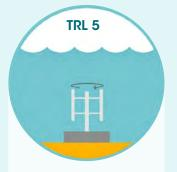
Vertical-axis turbine The tidal currents flow through a set of blades parallel to a rotating shaft, generating power irrespective of the direction of the flow.
