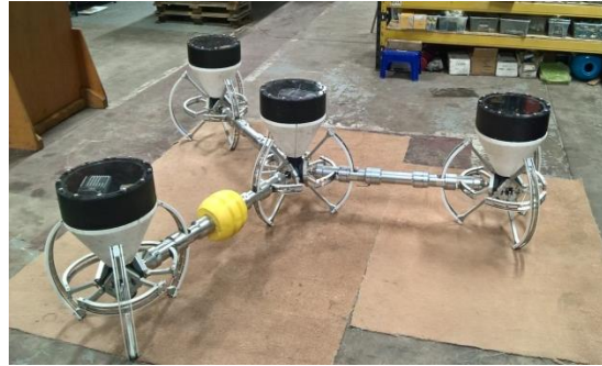
Albatern – Point Absorber/Attenuator
