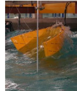
Zyba – Floating Surge Converter
