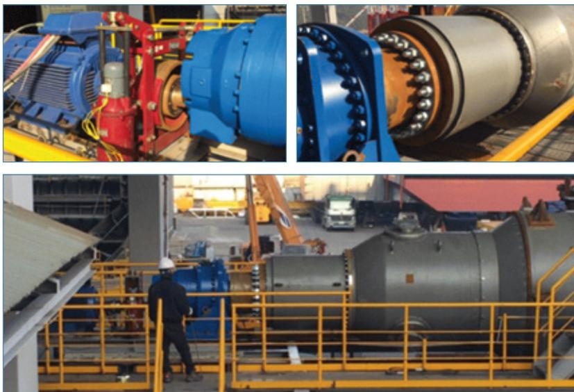
*Dynamo test for PMSG and drive train of 200 kW TEC*
