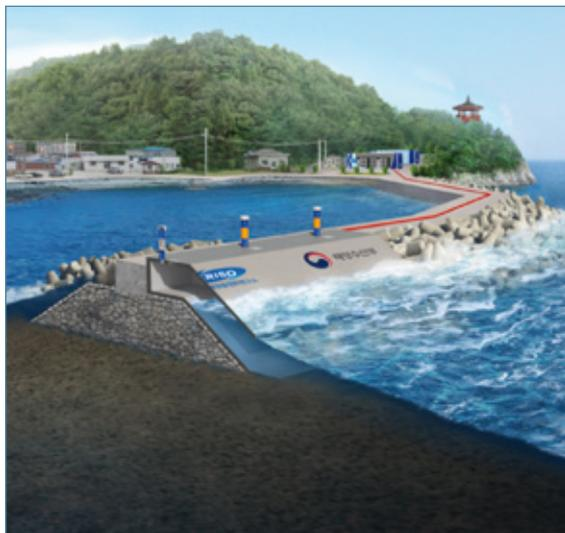
*WEC applicable to breakwaters on remote island*
