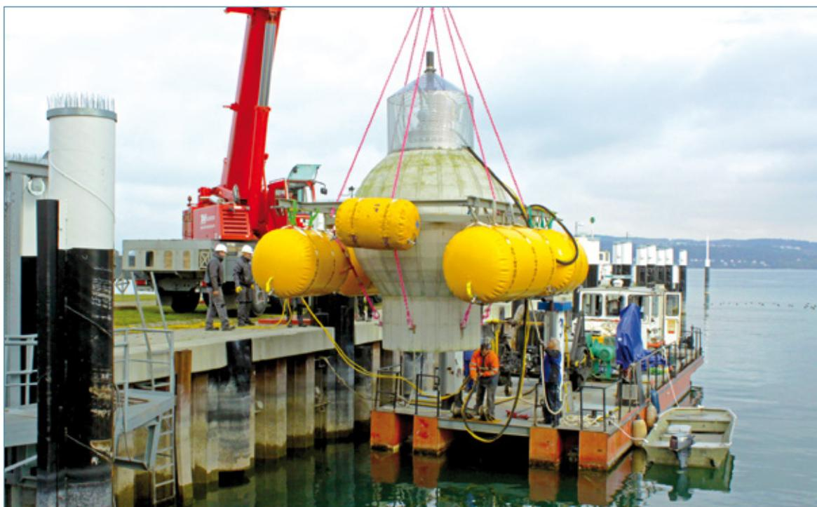
*“Stored Energy in the Sea” - 1:10 scale model tested in Lake Constance, Germany*
