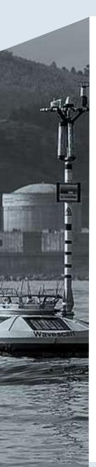
**Zunibal** — Anteia AP 2016/18 Wave measuring buoy
