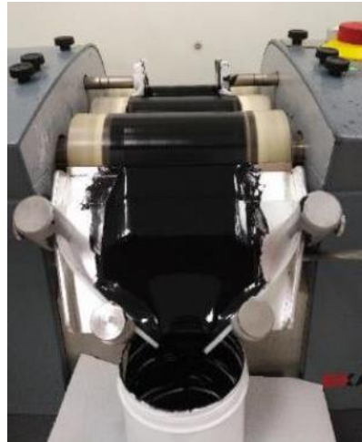
Dispersion of the CNT inside NEMMO resin at 2,5wt% using three rolls mill
