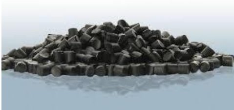
Commercial pellets (25wt% of CNT inside matrix)
