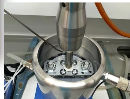
FUNDITEC's Set-up of cavitation erosion test
